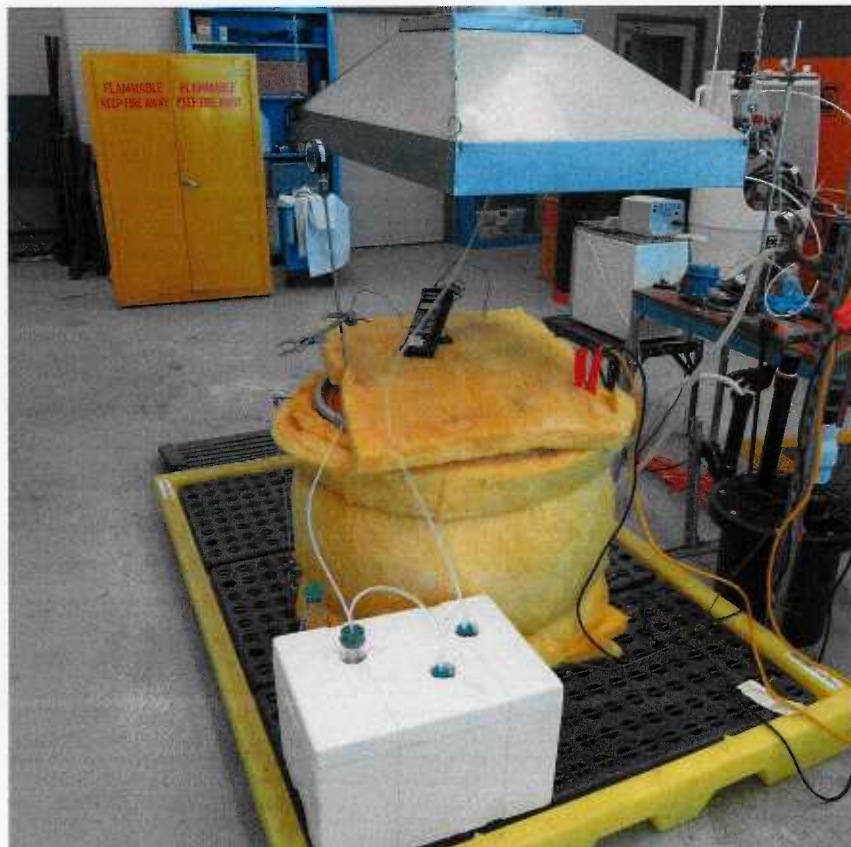
Figure 1. Test apparatus used to test vapor sealing properties of tiles.
