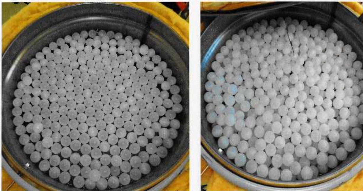
Figure 3. Picture showing ECC, LLC PVDF evaporation balls with one layer (left) and two layers (right) of balls.
