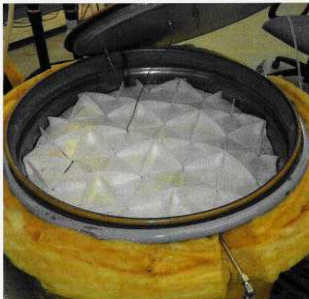
Figure 2. Picture showing placement of tiles on the surface of the toluene.
